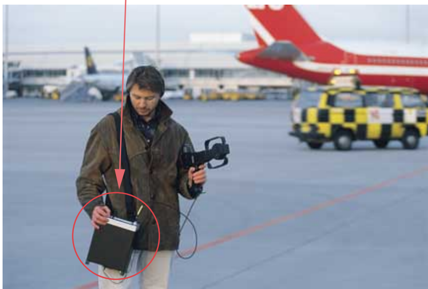
Removal of receiver from rack and use as a portable monitoring station
